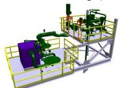
Issued For Construction (IFC) engineering data for all disciplines required for the construction of a single module. A group of modules (<10) is a single CWP. The steel and pipe EWPs for a CWP of modules becomes discrete fabrication packages that identify all of the spools and steel piece marks for the CWP (group) of modules.
